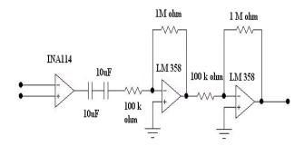
Figure 1 ECG data acquisition and amplifier circuit
