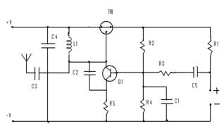
Figure 2 Circuit diagram of FM transmitter
