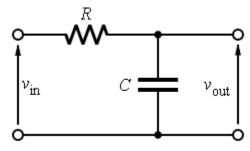
Figure 3 RC low pass filter
